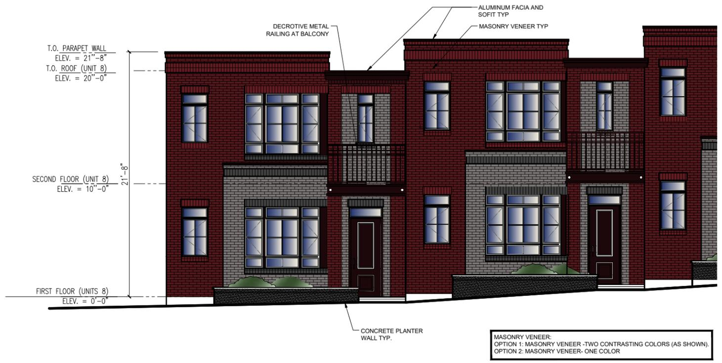
**2** SCHEMATIC SOUTH ELEVATION (PARTIAL)
